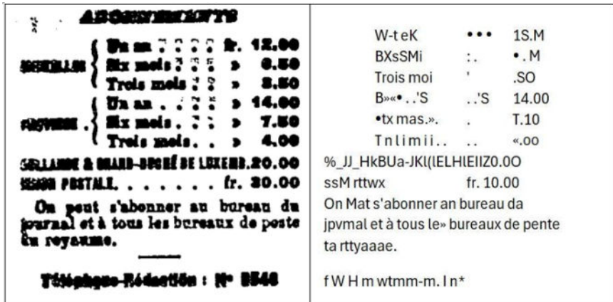
Fig. 2. Le XXe Siècle , issue of December 1, 1898, p. 1: comparison of the scan and the output of the OCR model for the subscription prices paragraph (the title and the two elements to the left of the braces were ignored by the OCR model).
