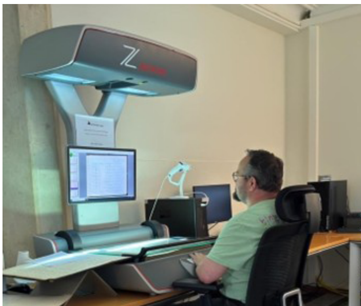
Fig. 2. Overhead A2 book scanner station for books that cannot be trimmed.
